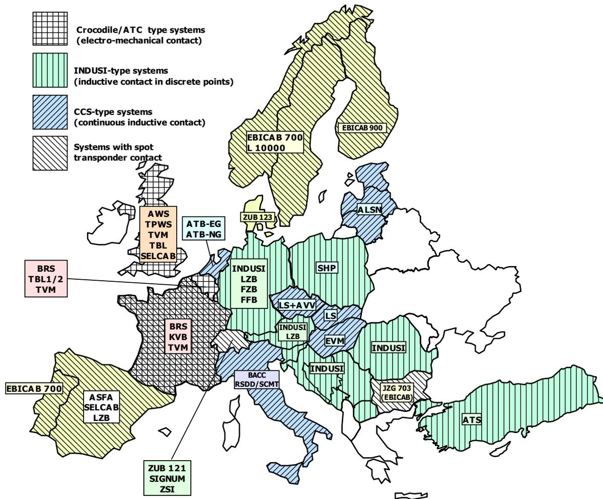
Fig. 2. Train control systems in Europe, without ERTMS/ETCS.
