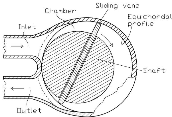
Fig. 8. Cutaway sketch of a trough vane rotary pump
