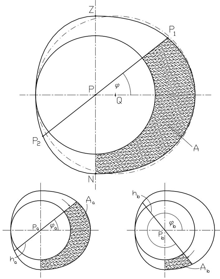
Fig. 10. The TCD curve and its basic feature elementary rotation of the shaft is):
