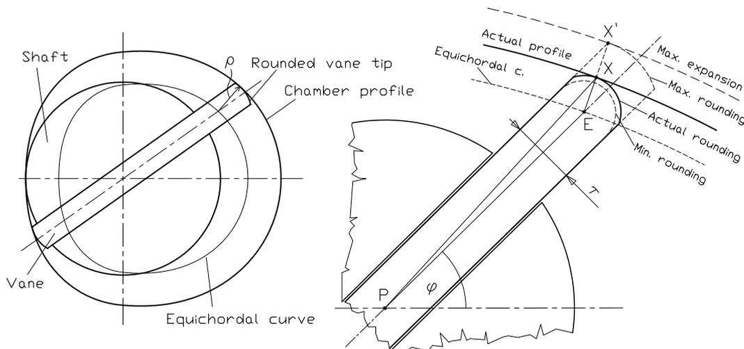
Fig. 9. Geometry of pump cavity having a realistic vane with rounded tips
