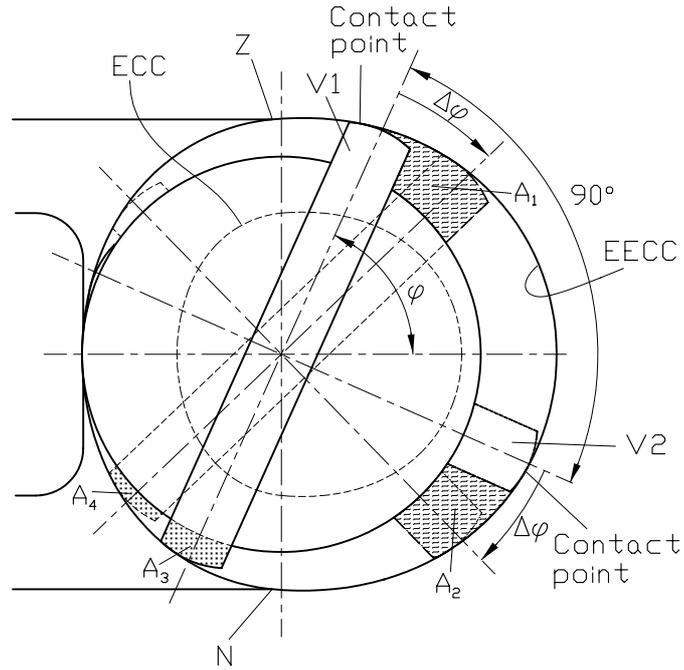
Fig. 11. Requirements for an RTCD curve taking into account the effects of the finite width of the vane
