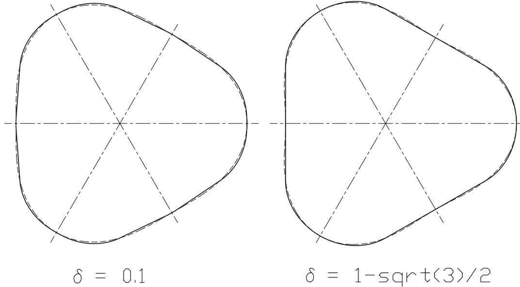
Fig. 7. Comparison of the critically convex 3-fold limaçon (dashed line) with the convex 3-fold TLPC ECC (continuous line) at  $\delta = 0.1$  and the critically convex 3-fold TLPC ECC (continuous line) with the nonconvex 3-fold limaçon (dashed line) at  $\delta = 1 - \sqrt{3}/2$
