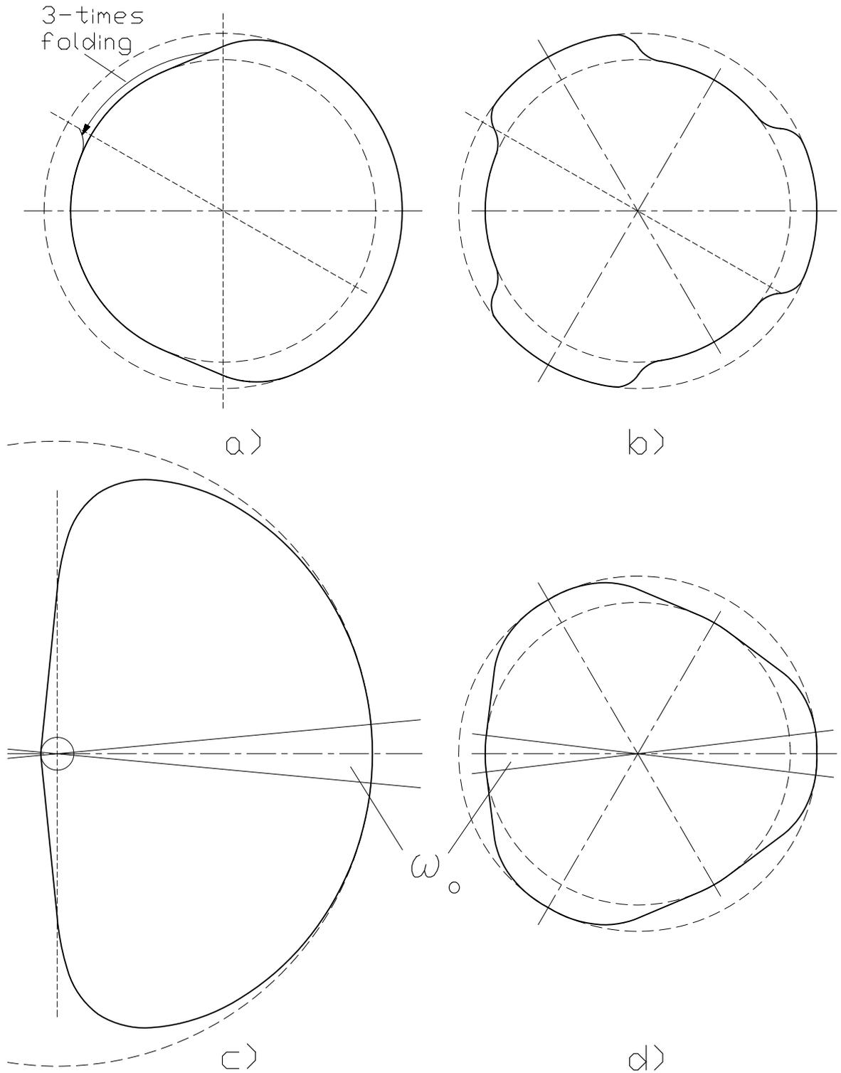
Fig. 6. Case b) is the 3-times folding of the TLPC ECC shown in case a) with a single symmetry axis, case c) is a 1-fold TLPC ECC having large eccentricity,  $\delta = 0.9$ , and case d) is a TLPC ECC with 3-fold symmetry. For cases a), b), and d)  $\delta = 0.08$ . Note that for cases c) and d), the  $\omega_0$  angles are roughly the same.
