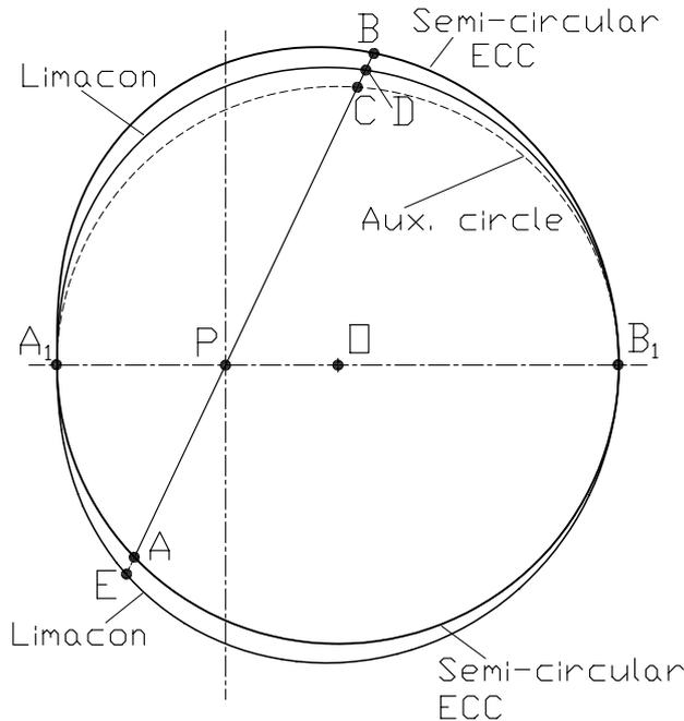
Fig. 3. Semi-circular equichordal curve and Pascal's limaçon
