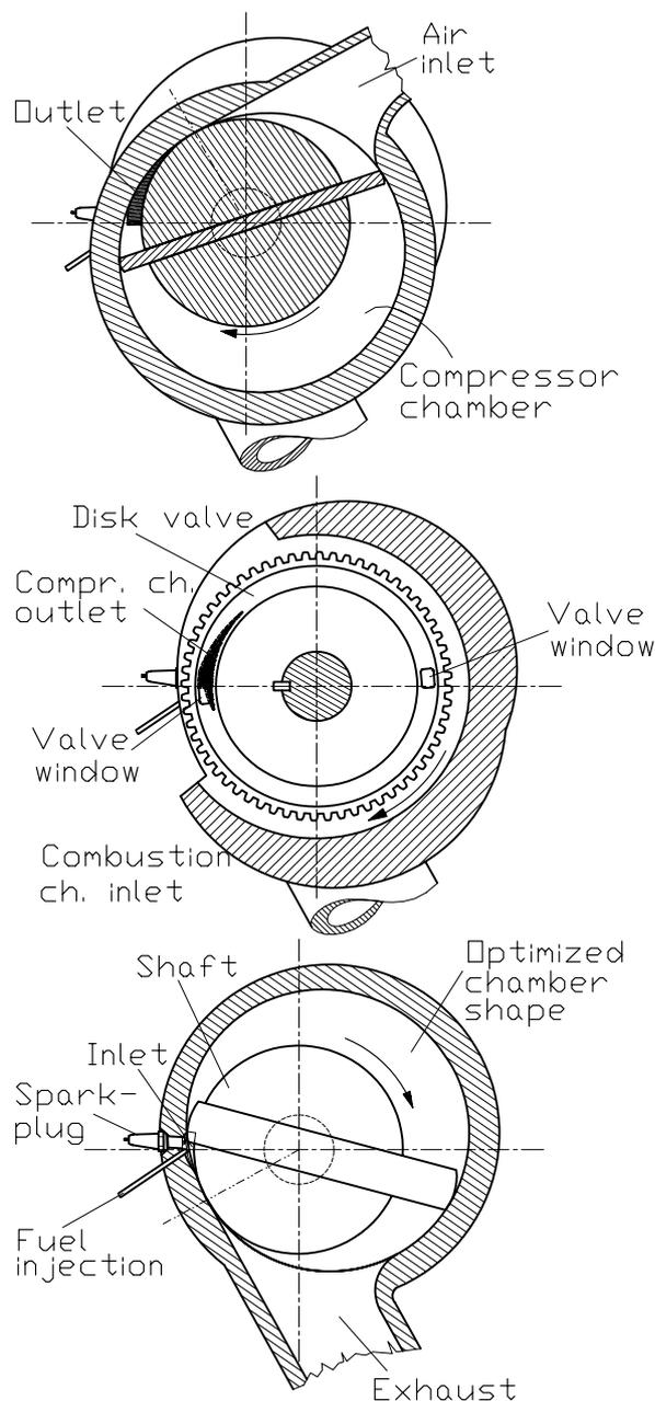
Fig. 12. Layout of a rotary internal combustion engine in three cross sections
